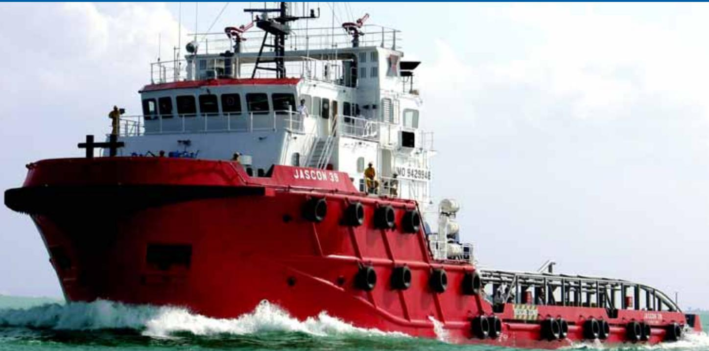
West African Ventures operates a large fleet of AHT / AHTS vessels varying between 35 and 75 m and 4000 and 8000 HP, most of which are equipped with DP-1 or DP-2 system.
